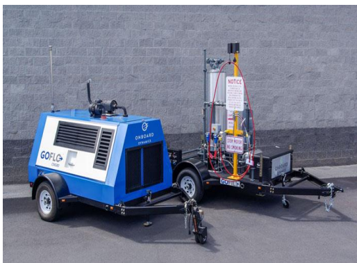
Natural gas compressor and Go-Flo instant fueling station
